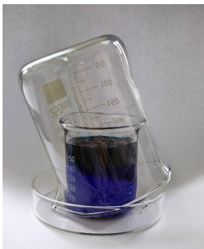
Fig. S15 Apparatus for the collection and purification of dye-containing wastewater.
