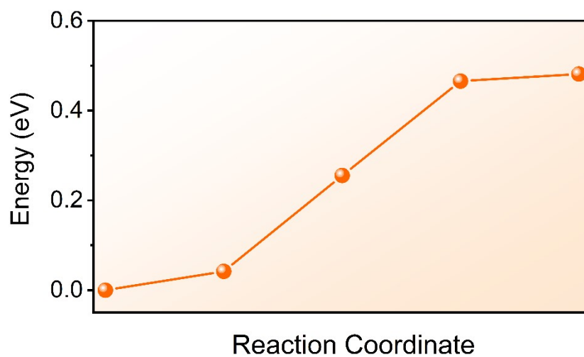
Fig. S5 The reaction energy for migration process of the V1- Br, where the initial and final state is V1- Br (dimmer-like) and V1- Br (unbound) structure, respectively.
