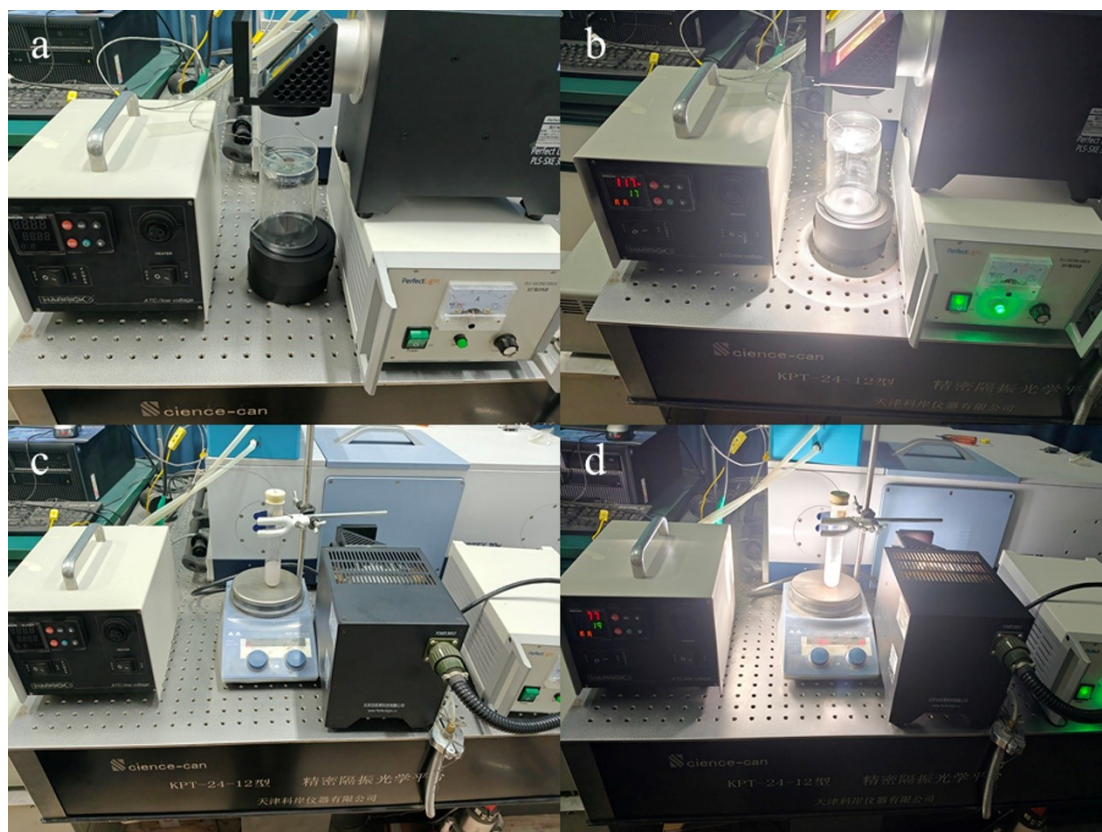
Fig. S5 The home-made equipment for measuring the temperature of the surface of catalysts and the solutions under Xe lamp irradiation.
