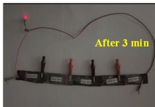
**Fig. S31** Picture showing individual potential of one device, series connection of five devices and illumination of LED (3.0V)
