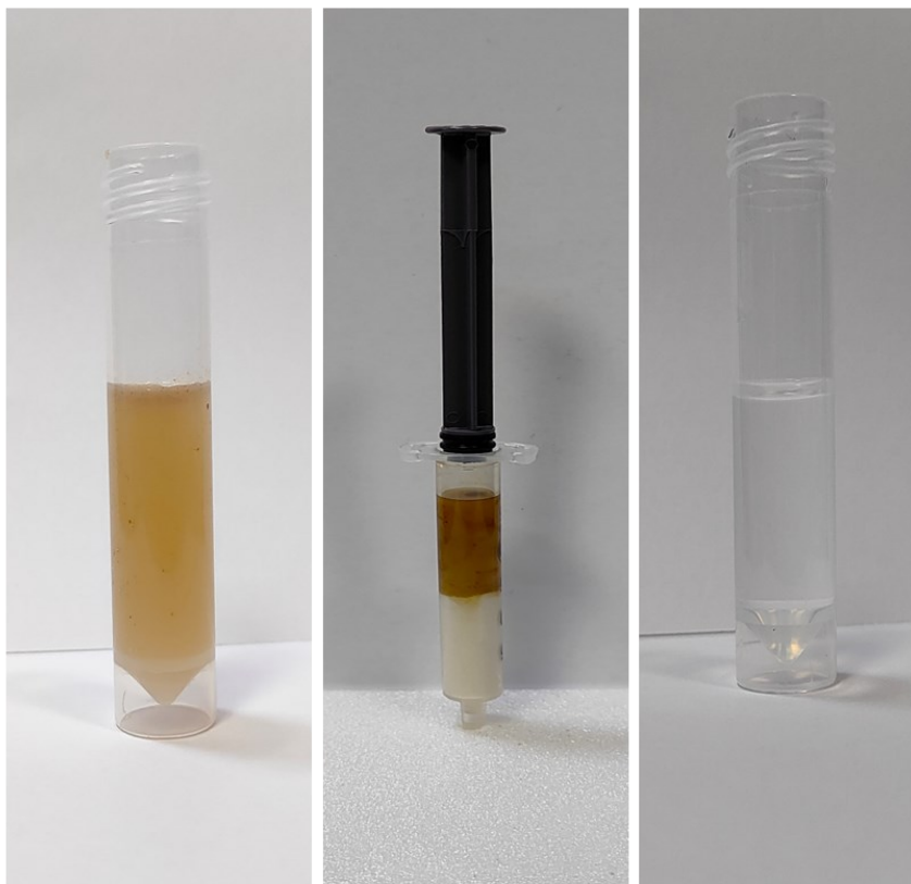
Figure S21. (a) Schematic diagram of oil/water emulsion separation with the Shola pith packed inside a syringe, (b) Image of laboratory experiment (crude oil/water emulsion , packed Shola pith with the emulsion, and eluted water).
