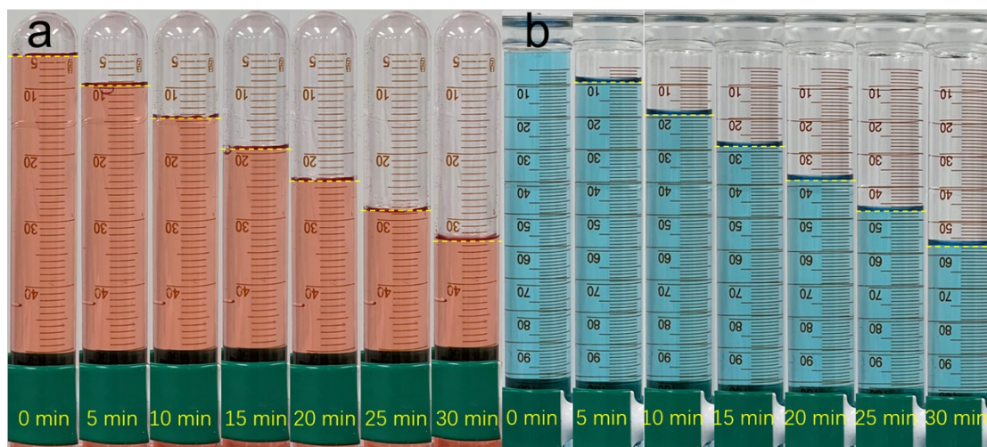
Fig. S20. The gas photographs of (a) O_2 and (b) H_2 varying with time at 1000 \text{ mA cm}^{-2} by drainage method in 1 \text{ M KOH} + \text{seawater} .
