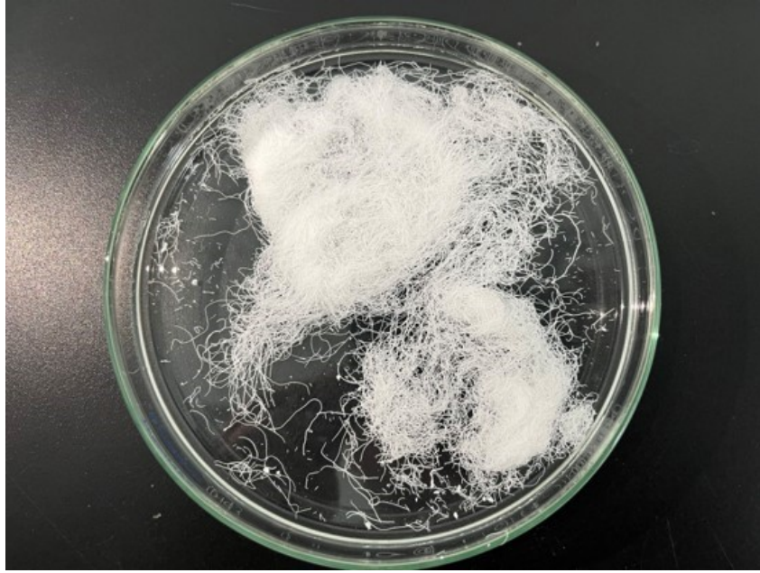
Figure S3. The digital image of fiber prepared by wet spinning.
