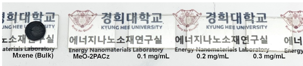
Figure S3. Photographic images of MXene (bulk), MeO-2PACz, MeO 2 PACz/MXene films with varied concentration of MXene deposition.
