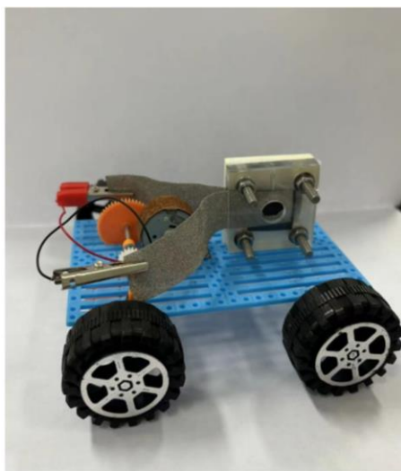
Fig. S38. A toy car powered by a Zn-air battery constructed with Co@N-CNT.
