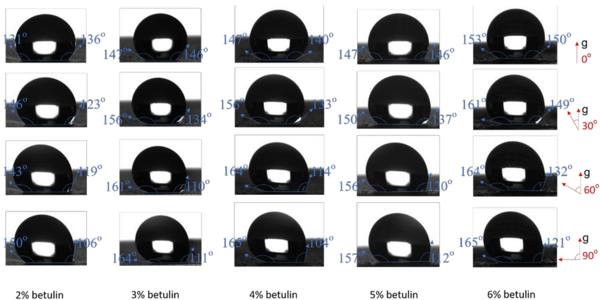
Fig. S2 Water drop (5 \mu l) pinning to the betulin-coated surfaces demonstrated through roll-off contact angles. Each column corresponds to a Bet-PLA-2 coating with betulin content displayed at the bottom. The red arrows on the right-hand side indicate the inclinations of the surface in the row.
