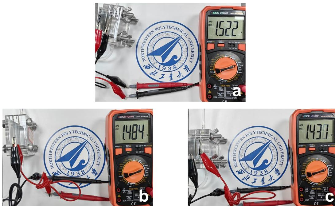
**Figure S18.** Digital photo of OCP measured by multimeter of ZABs using (a) Co-Pt@Fe-N-C, (b) Pt@Fe-N-C and (c) Pt/C as catalysts.
