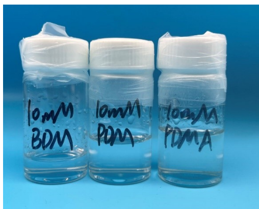
Fig. S1. Optical photo of 2 M \text{ZnSO}_4 electrolytes with 10 mM BDM, 10 mM PDM and 10 mM PDMA after preparation for 6 months.
