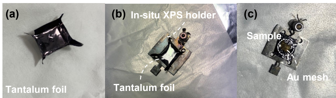
Fig. S2. (a) Tantalum (Ta) foil. (b) The in-situ XPS holder was welded with Ta foil. (c) The four sides of the holder can be folded to accommodate and secure the Au mesh.
