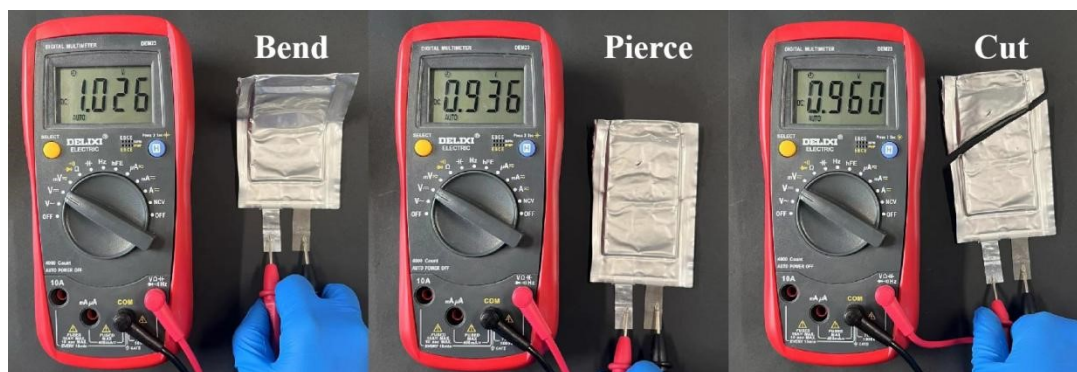
Figure S11. Pictures of voltage changes in Zn||PANI solid-state soft-pack batteries under bending, piercing, and cutting.
