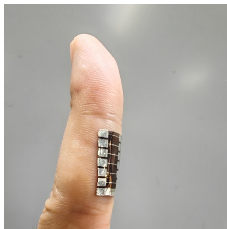
Fig. S18. Photograph of the free-standing OPVs attached to a finger.
