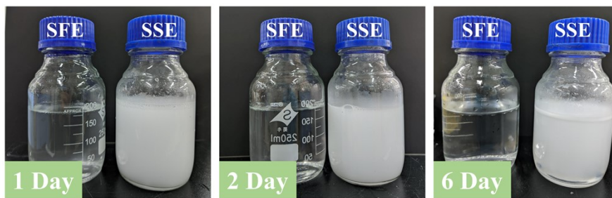
Fig. S4. Digital photographs of as-prepared SFE and SSE during a 6 day placement.
