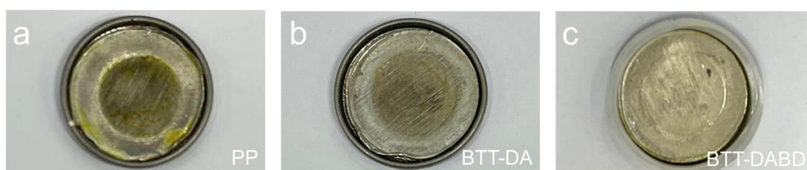
Figure S22. Photographs of cycled Li anodes for (a) PP, (b) BTT-DA, and (c) BTT-DABD separators, respectively.
