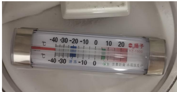
Figure S6 The thermometer placed in the low-temperature freezer for 1h indicates a stable internal temperature of -40°C.
