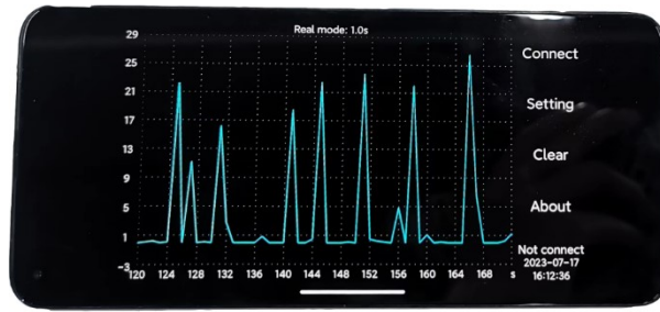
Figure S20. Wrist flexion current display on a smartphone.
