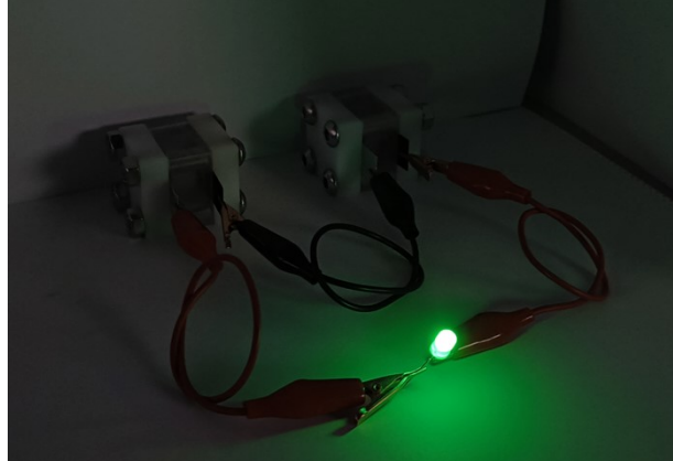
Fig. S16. A lighted green light-emitting diode (LED) powered by two series of homemade ZAB with C@Ir/CNF1000: (a) operation video, (b) digital image.
