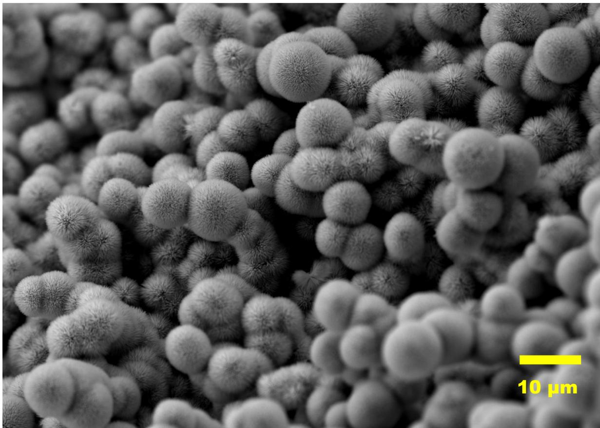
**Figure S2:** SEM image of the  $\text{NiCo}_2\text{O}_4$  precursor
