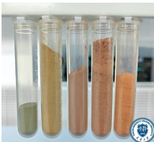
Fig. S1 Optical photos of the precursor, from left to right, show NiFe, Mo 0.25 -NiFe, Mo-NiFe, Mo 0.75 -NiFe, Mo 1.0 -NiFe.
