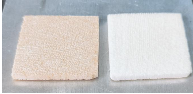
Fig. S14: WA has high reflectance in the visible light range, showing a bright white appearance (right). Natural wood contains lignin, which can absorb visible light, thus showing a yellow appearance (left).
