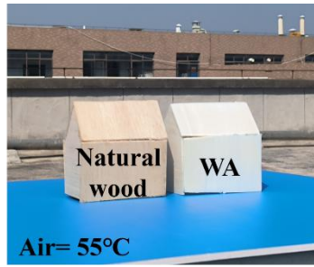
Fig. S23: The two houses are constructed with natural wood and WA respectively, and are positioned outdoors where the environmental temperature is 55°C.
