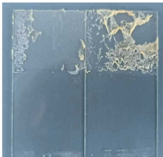
Figure S11. Image of PSLTP as a detachable adhesive after lap shear experiment.
