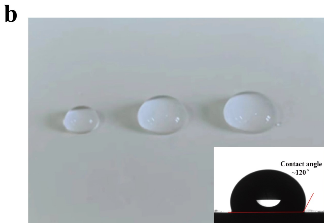
Figure S10. SM film are tested for hydrophobicity with various liquids. (a) Hydrophobicity test conducted with four different liquids (cola, fanta, milk and water) and the sample moulds. (b) Hydrophobicity test performed with different volumes of liquid and sample mould.
