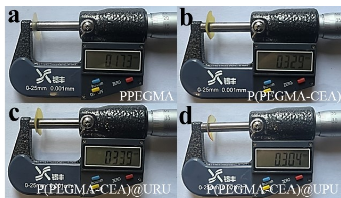
Fig. S14 Thickness of SPE membranes.
