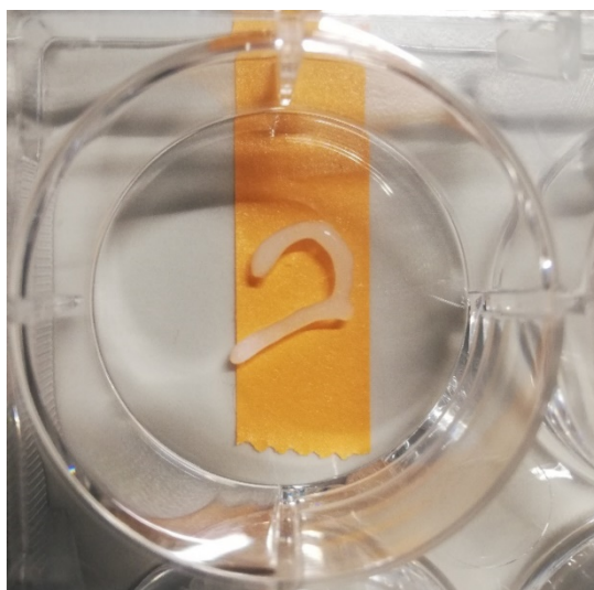
Fig. S6. Injectability of NBTA-MSN 1 nanocomposite hydrogels through the 19-Gauge syringe needle
