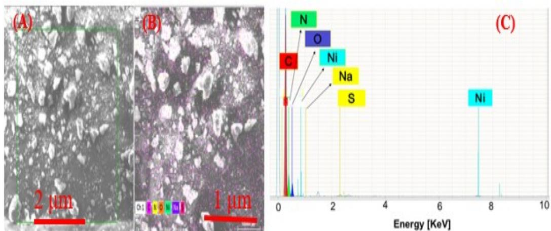
**Figure S2:** A and B SEM and C EDX pattern of KL@Ni@g-C<sub>3</sub>N<sub>4</sub> hybrid composite.
