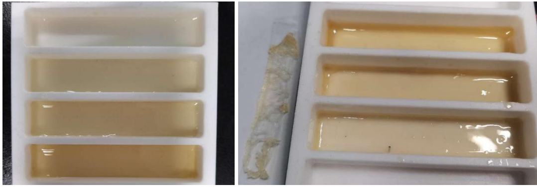
Figure S5. Tape that was blocked from polymerization by tannic acid in the pre-experiment
