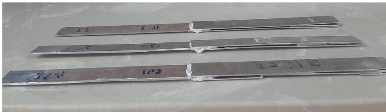
Fig. S5. Side view of double overlap adhered samples prior to testing
