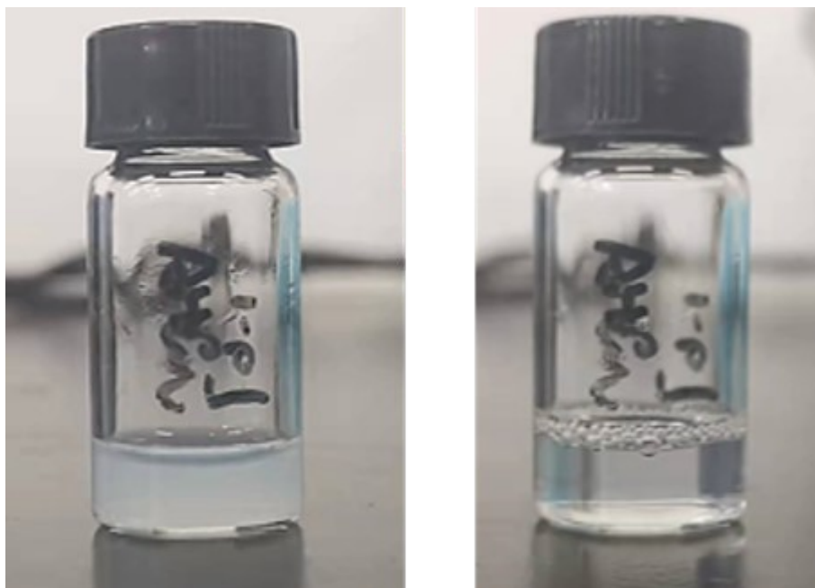
Figure S7. Responsiveness of AHCu in the presence of GSH (left: AHCu; right: AHCu + 2mM GSH).
