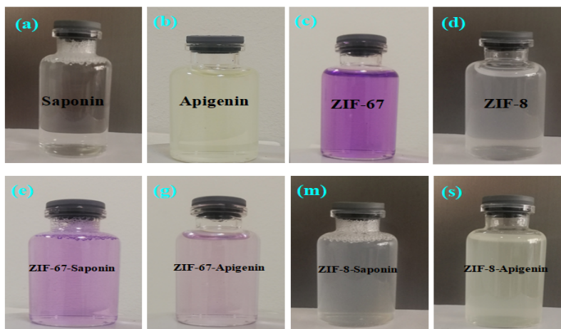
Figure S2. The bottom figures nanoparticles with natural products prepared are shown. (a) saponin, (b) apigenin (c) ZIF-67, (d) ZIF-8, (e) ZIF-67-Saponin, (g) ZIF-67-Apigenin, (m) ZIF-8-Saponin, (s) ZIF-8-Apigenin.
