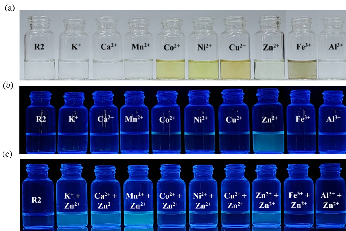
Fig. S11 Visual responses of R2 upon addition of different metal ions under ambient (a) and UV light (b) conditions, and towards \text{Zn}^{2+} cation in the presence of various competing metal ions under UV light condition (c), in \text{CH}_3\text{CN}:\text{DMSO} (v/v 9:1).
