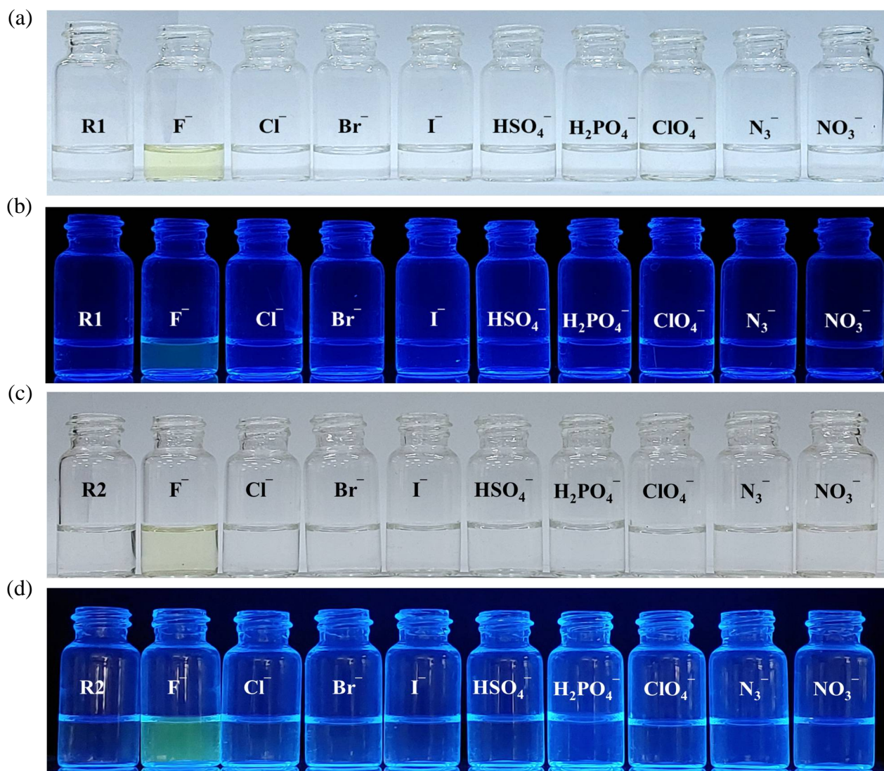
Fig. S14 Visual responses of R1 upon addition of different anions under ambient (a) and UV light (b) conditions, and R2 upon addition of different anions under ambient (c) and UV light (d) conditions, in CH 3 CN:DMSO (v/v 9:1).
