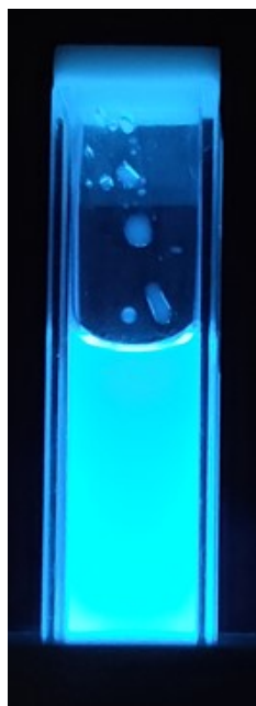
Fig. S3. Blue fluorescence of E_2 -CA-CD observed under UV torch irradiation (excitation 365 nm)
