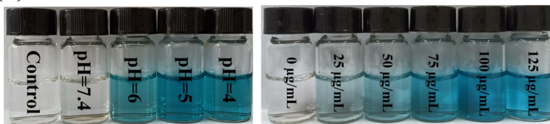
Figure 2S. (A) Digital photographs of oxidase-like activity of H-MnO 2 , the effect of pH and concentrations on the oxidase-like activity. (B) Imaging for peroxidase-like activity of H-MnO 2 , the effect of pH and concentrations on the peroxidase-like activity.
