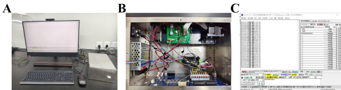
Fig. S3 (A) The appearance photo of the portable fluorescence reader with the matching computer. (B) The internal structure photo of the portable fluorescence reader. (C) The main interface of the fluorescence signal processing software.
