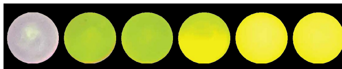
Figure S3. Images of fluorescence responses of TLC plates impregnated with BOPD (200 \mu\text{M} ) upon exposure to various concentrations of phosgene gas (left to right: 0 ppm, 0.1 ppm, 5 ppm, 10 ppm, 30 ppm).
