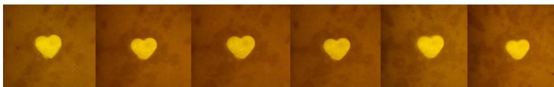
Figure S13. The stability and durability test were conducted for “heart” pattern visualized with CA-CB[7] system under the repeated rinsing procedure. The “heart” pattern was washed with pure water for 6 times. And the fluorescence pattern was imaged with photography after rinsing every time.
