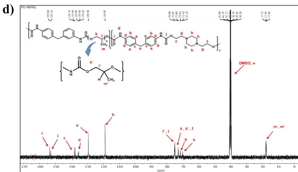
Fig. S4: ^{13}\text{C} NMR spectra of a) PU1, b) PU2, c) PU3, and d) PU4.
