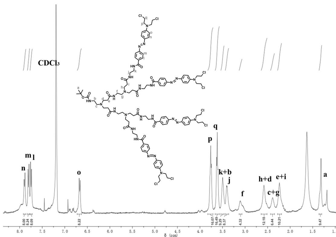
**Fig. S2** <sup>1</sup>H NMR spectra of Boc-D2-Azo-CB<sub>4</sub> (CDCl<sub>3</sub>).
