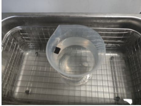
Figure S2. The foam was ultrasonically cleaned in deionised water.
