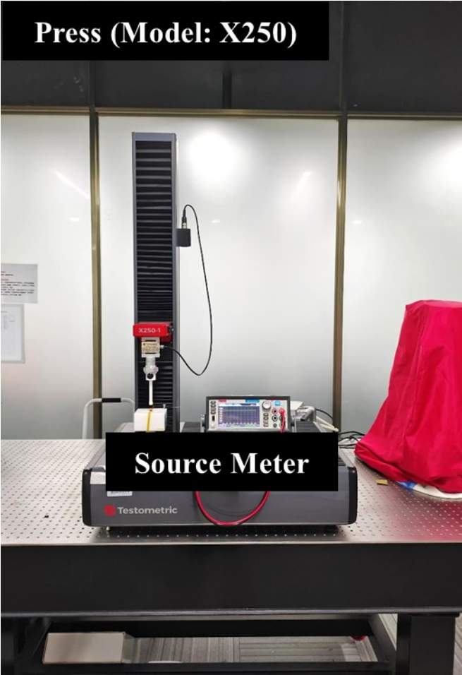
Figure S3. Photograph of Testometric material testing system.
