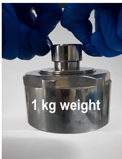
Fig. S2 Load lifting capability of [\text{Gel}_{10}](\text{AmAc}_{55}\text{AmC}_5) hydrogels, indicating excellent mechanical toughness.
