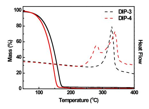
**Figure S1.** thermogravimetric analysis (TGA, solid line) and differential scanning calorimetry (DSC, dashed line) of the two precursors. These precursors are almost vaporized at 150°C. DIP-3 (black) shows one heat flow on 320°C, but DIP-4 (Red) shows two heat flow point at 250°C and 330°C.
