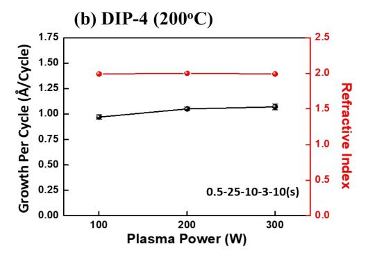
**Figure S2.** ALD process optimizing of In2O3 PEALD using DIP-3 and DIP-4. (a) plasma time for DIP-3, (b) plasma power for DIP-3, (c) plasma time for DIP-4, (d) plasma power for DIP-4
