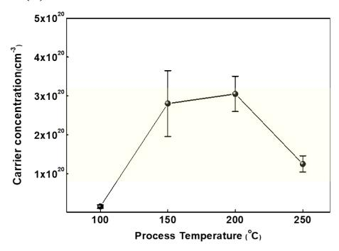
**Figure S3**. Carrier concentration variation in the Hall measurement result. (a) DIP-3 (range:  $1 \times 10^{20} \sim 5 \times 10^{21}$ ) (b) DIP-4 (range:  $1 \times 10^{19} \sim 5 \times 10^{20}$ )
