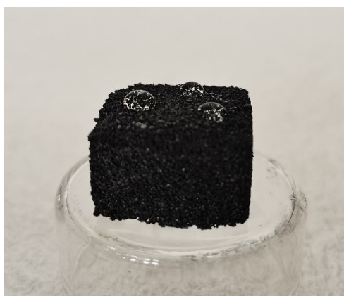
Figure.S8 Photos of water droplets on the surface of rGO@GA/PDMS composite material
