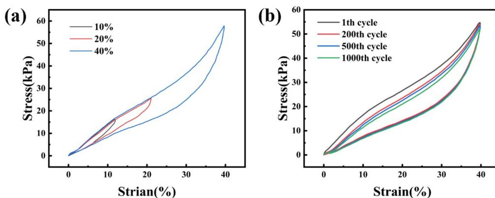
**Fig. S6.** The compressive stress-strain curves of rGO@WS. (a) Compressive stress-strain curves at different strains of 10, 20 and 40%. (b) Compressive stress-strain curves at 40% strain for 1000 cycles.
