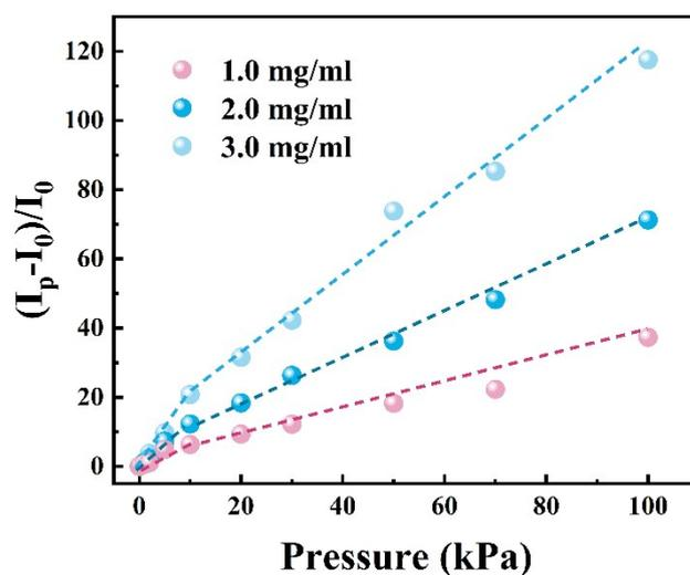
Fig. S4. The sensitivity curves of rGO@WS sensors under different rGO content.
