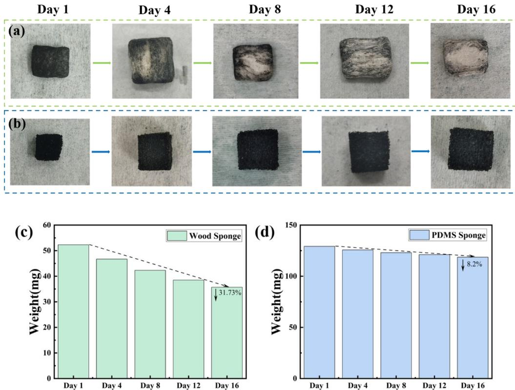
**Fig. S13.** The appearance of (a) wood sponge, (b) PDMS sponge during the degradation process. The weight of (a) wood sponge, (b) PDMS sponge during the degradation process.
