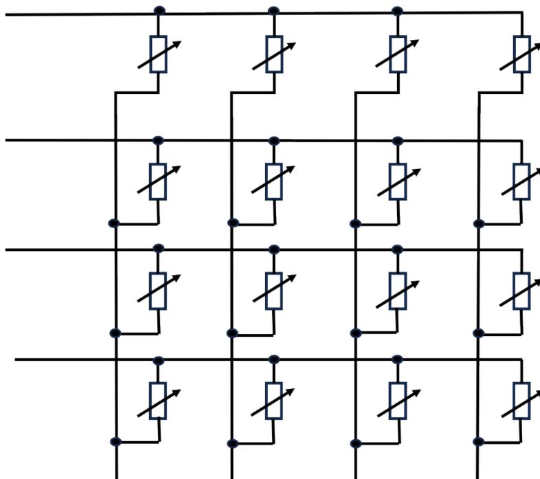
**Figure S9.** The equivalent circuit diagram of this pressure array.
