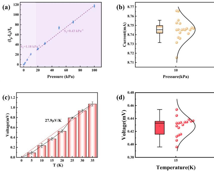
**Fig.S12.** The error analysis of pressure and temperature performance. (a) Repeated measurement of the sensitivity curve with error bar. (b) Repeated measurement of the generated current under 10kPa. (c) Repeated measurement of the seebeck coefficient with error bar. (d) Repeated measurement of the generated voltage under 5K.
