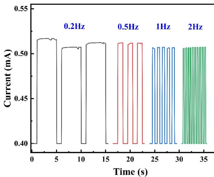
Fig. S7. The frequency-independent stability of rGO@WS.
