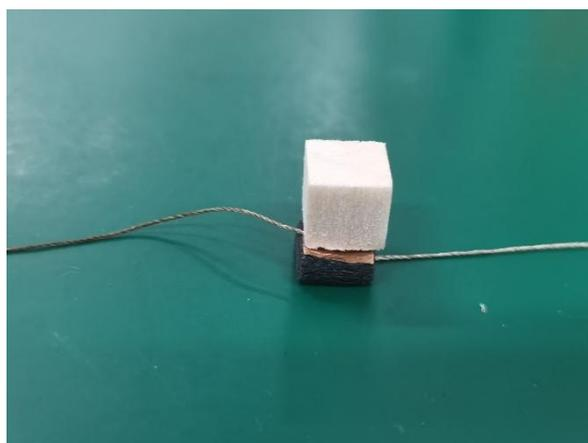
**Figure S5.** The minimal detection limit tested by a light wood.
