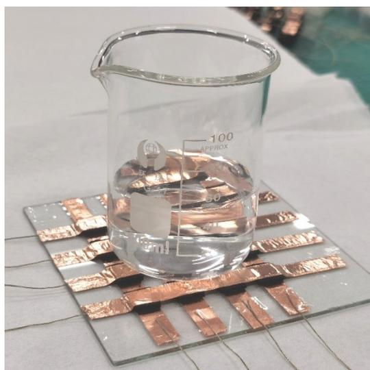
**Figure S10.** The pressure and temperature test of the rGO@WS sensing array.
