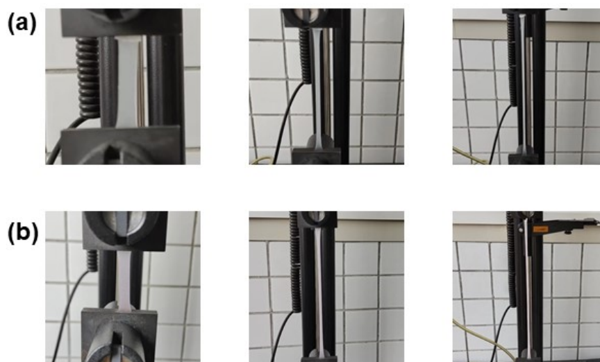
Fig. S7 Stretching changes of (a) SIS-SPM 1 -UPy and (b) SIS-SPM 2 -UPy
