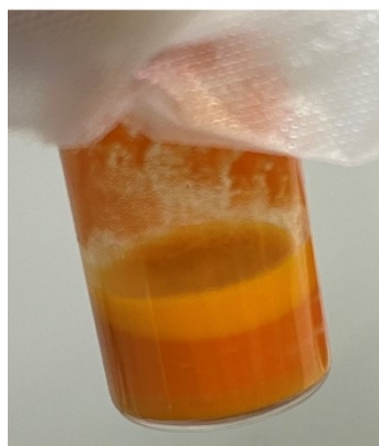
Fig. S5 \text{Cs}_2\text{AgBiBr}_6 single-crystal powders were dispersed in ACN, yielding a viscous suspension.
