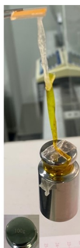
Fig. S8 The \text{Cs}_2\text{AgBiBr}_6 thick film with 30 \text{ mg mL}^{-1} SO. A 100 g weight is attached to the surface of the film via PI tapes.
