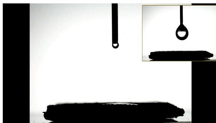
Figure S9. Contact angle measurement's image of ZCR-3 NCs-based photoanode (inset: image before water contact).
