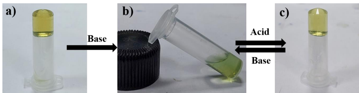
Figure S13. (a) Hydrogel before exposure to pH change, (b) increasing pH by adding base leading to gel to sol transition of the hydrogel with bluish colour, and (c) acid added to the previous system to lower pH leading to restoration of the gel.
