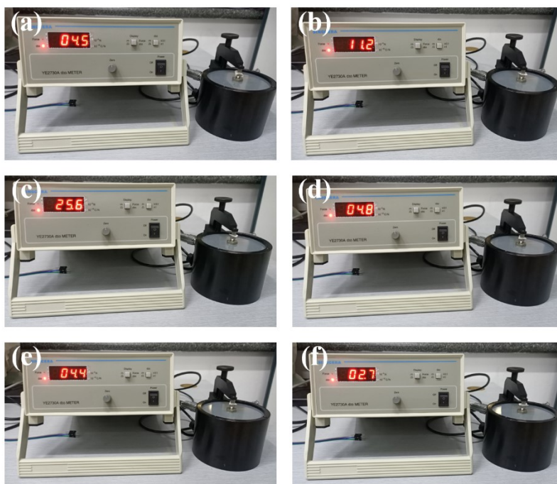
Fig. S8 Piezoelectric constant ( d_{33} ) of (a) pristine cotton, (b) SCF-0.5, (c) SCF-1.0, (d) SCF-1.5, (e) SCF-2.0 and (f) SCF-2.5 measured by a commercial d_{33} meter.
